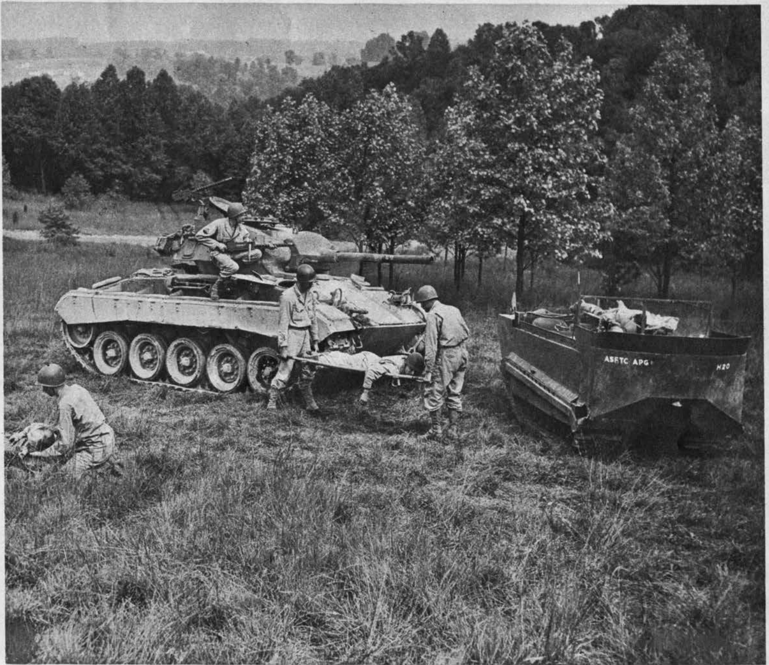
New light tank is the low, powerful M-24. Its angular turret has a two-inch M-3 mortar, a 75-mm. cannon and two machine guns. The low, wide silhouette and modified Christie suspension are typi-
